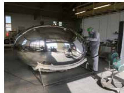
The pendulum, a handcrafted unique piece made of driven aluminium, has the shape of an egg. Its small diameter is 1.5 meters, the larger 3 meters. The surface was polished by hand in an elaborate process.
